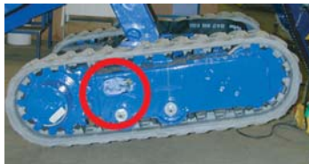
Fig. 66a The nipples for the tension roller is placed here
