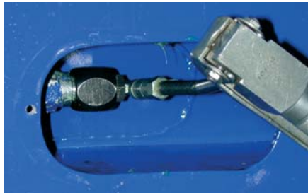
Fig. 67a Grease gun on grease nipple with adaptor for the tension roller
