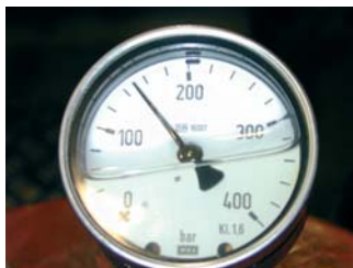
Fig. 68a Pressure gauge on Grease gun
