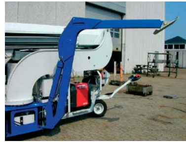
Fig. 12 Outrigger turned away from the platform
