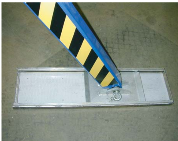
Sliding track mounted at the outriggerAppendix B: Key switch at the turret
