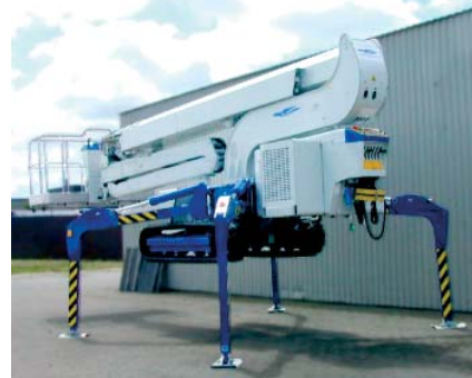
Fig. 58 Platform lifted at the outriggers
