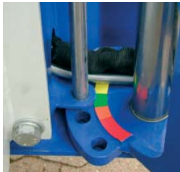
Fig. 17 Outrigger in standard position.
